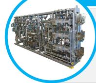
Gas seal panels, according to ISO 10438:2008 Part 4 and API 614 Fifth Edition Chapter 4, are designed to supply seal and buffer gas to the shaft seals. They include filters, controls, piping or tubing and the related instruments and cover a wide array of flows, pressures and material grades.
